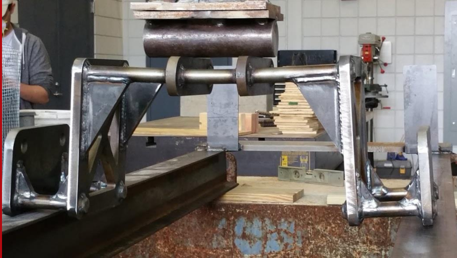
Trolley + Gantry under 2500 lb. load
